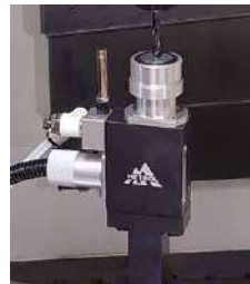
Tool length switch for automatic measurement
