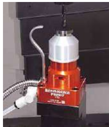
Tool length switch for automatic measurement
