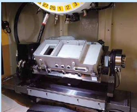
Example of indexing application by DDR-TiB
